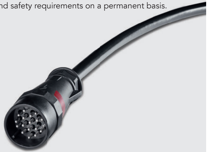
UIC 558 plug: Red color markings for 18-pole version
